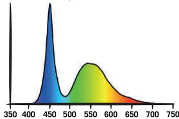
The 6500 Cosmorrow LED light, made up of "White 6500 °K" LEDs, is designed for the vegetative, cutting or growing stage. We recommend placing it as close as possible to the plants, as its surface temperature is low.
