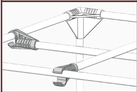
The HANDLING TUBE allows you to install lighting and ventilation wherever you want. There are two hooks in the corners so two bars can easily be stacked on top of each other without getting in the way. This system also allows two parallel bars to be positioned at exactly the same height. These tubes can support from 10 to 25 kg on a single bar, depending on the tube's diameter.
