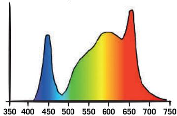
The BLOOM Cosmorrow LED, also called the Full Spectrum light, is designed for blooming and fruiting, with a red peak at 660 nm. The blue peak at 440 nm also makes it suitable for cutting and growing. We recommend installing it at a distance of 15 to 35 cm from your plants.
