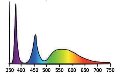
The UV Cosmorrow LED consists of 33% near ultraviolet (365 nm) and 66% 6500 °K LED (cool white). It is designed for growing, fights mould growth and improves plants' immune systems. UV light can damage plants if they are exposed to it for long periods.
