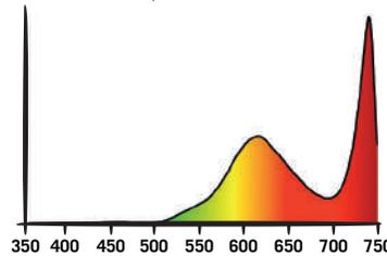
The IR Cosmorrow LED light consists of 33% near infrared light (730 nm) and 66% 2100 °K LED light (warm white). It is designed for blooming and fruiting, it also acts as a radiant heater that helps sun-loving plants to grow tall.
