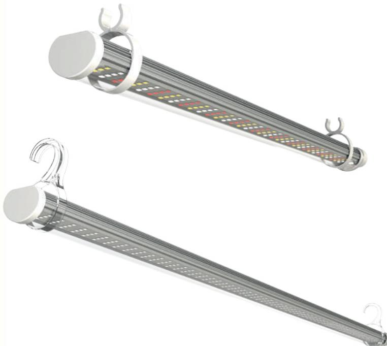
TLED is a 220 volt LED light with a very long life (up to 50,000 hours). It comes in two wattages - 26w / 21.3 inch and 42w / 37.5 inch - and two "colours" - Grow and Bloom, also called Full Spectrum. It is ideal for low plants and can also be used as a complement to a lighting system by clipping onto the vertical poles of your grow room.
